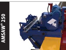
Special dual rail saw for field service, mounted to rail car.
