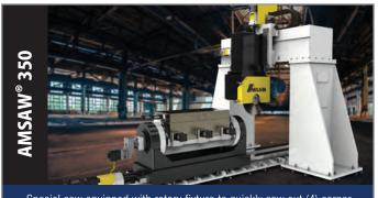
Special saw equipped with rotary fixture to quickly saw out (4) corner sections of valve bodies, instead of a time consuming milling process.
