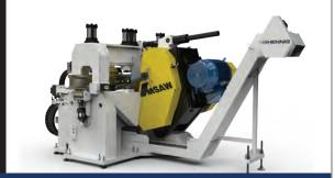
Heavy duty pivot saw to cut alloy rails.
