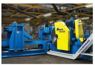
**AMSAW 760** MAX BILLET SIZE 760 MM (30") Complete with 1,000 mm (40") automatic measuring unit and Henniq chip conveyor.
