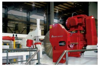
**AMSAW 450** MAX BILLET SIZE 450MM (18") Horizontal, heavy duty, carbide slide saw for hard alloy steel.
